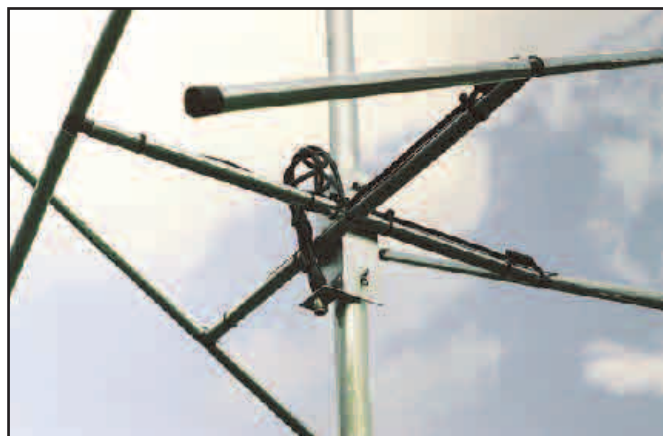
Figure 3 — View of cross booms mounted to mast.
